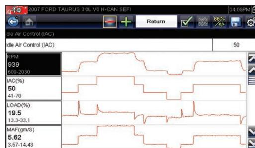
Use bi-directional controls while viewing live data for true cause and effect diagnostics.
